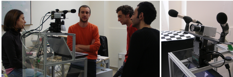
Figure 9.1: On the left: an example of the robot following a conversation in the Lab. On the right: the robot head with a pair of microphones and a camera oriented by a pan-tilt unit.
